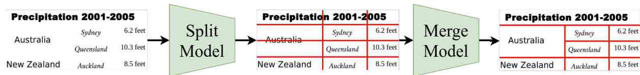
Figure 7.1: Overview of the proposed models. First the Split model predicts the grid of the table. Then the merge model combines grid elements to recover spanning cells.
