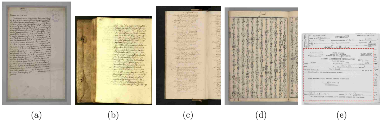
Figure 5.1: Examples of common border noise. (a-d) Background around the border. (b-d) Book edges. (c-d) Textual noise due to neighboring pages. (e) Textual noise due to one document (red square) overlaid on top of another.
